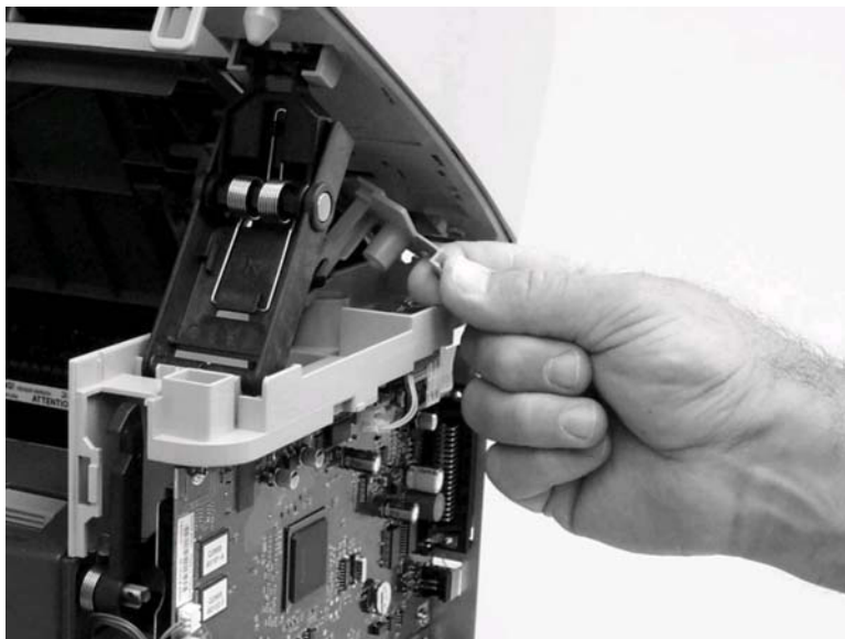
Figure 5-33. Remove the scanner assembly (10 of 15)
