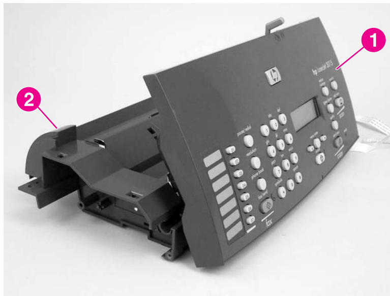
Figure 5-45. Remove the top-cover assembly (1 of 2)
