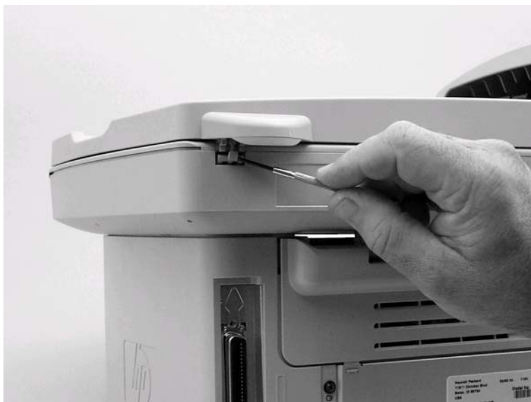
Figure 5-56. Remove the flatbed lid (3 of 5)
