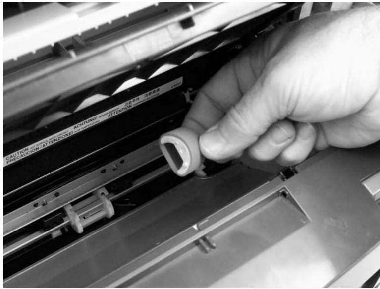
Figure 5-95. Remove the printer pickup roller (3 of 5)
