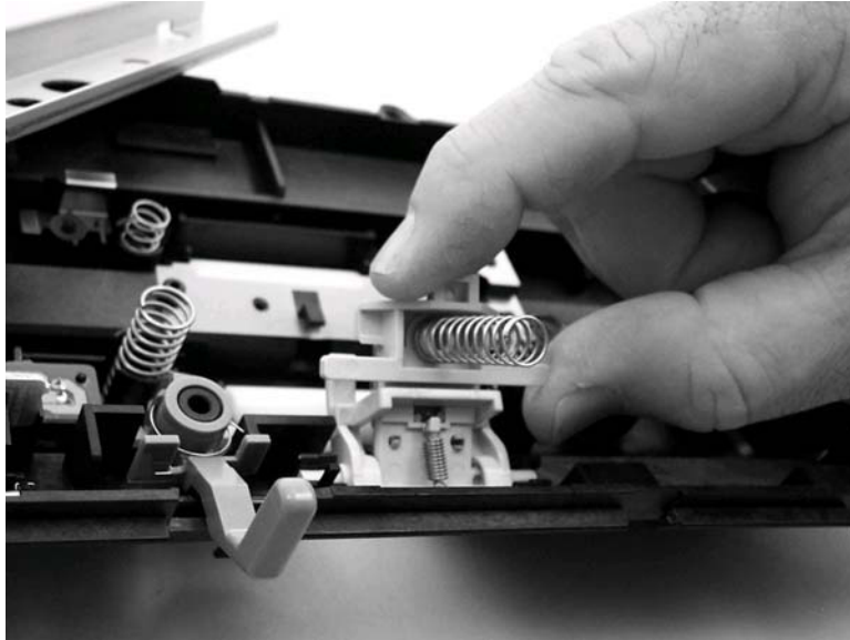
Figure 5-22. Remove the separation pad assembly (2 of 3)
