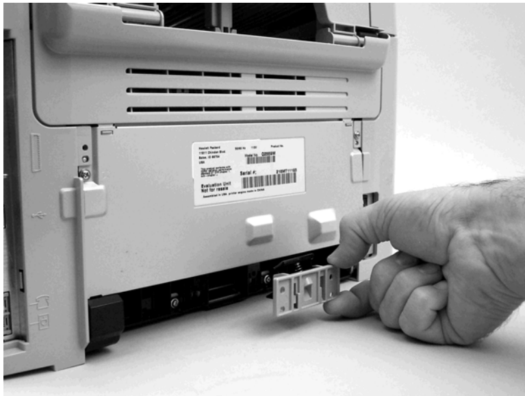
Figure 5-90. Remove the printer separation pad (2 of 2)
