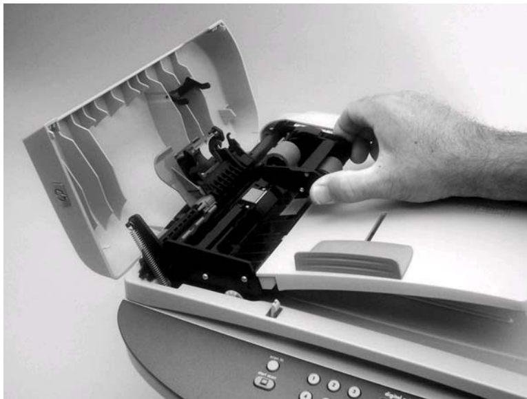
Figure 5-70. Remove the ADF pickup roller (2 of 2)
