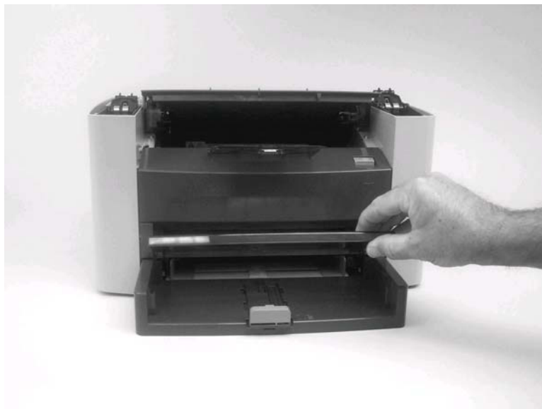
Figure 5-98. Remove the media input tray (1 of 3)
