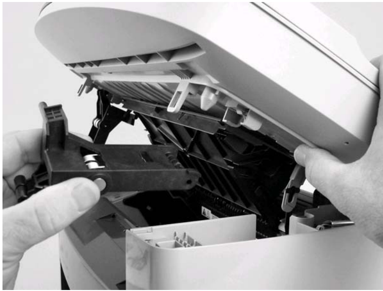
Figure 5-61. Remove the link assemblies and scanner support frame springs (3 of 4)
