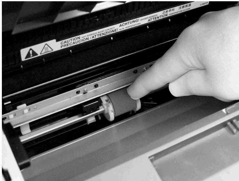
Figure 5-97. Remove the printer pickup roller (5 of 5)
