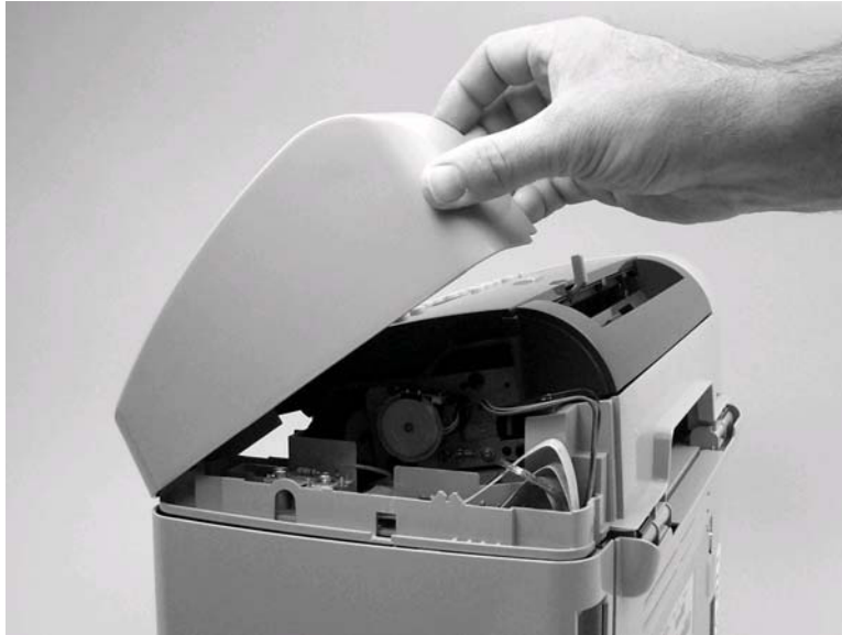
Figure 5-12. Remove the scanner side covers (3 of 3)
