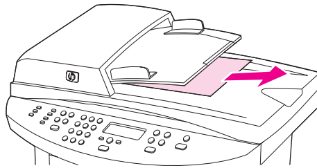
Figure 6-7. Clearing output bin jams (HP LaserJet 3020 and 3030)
