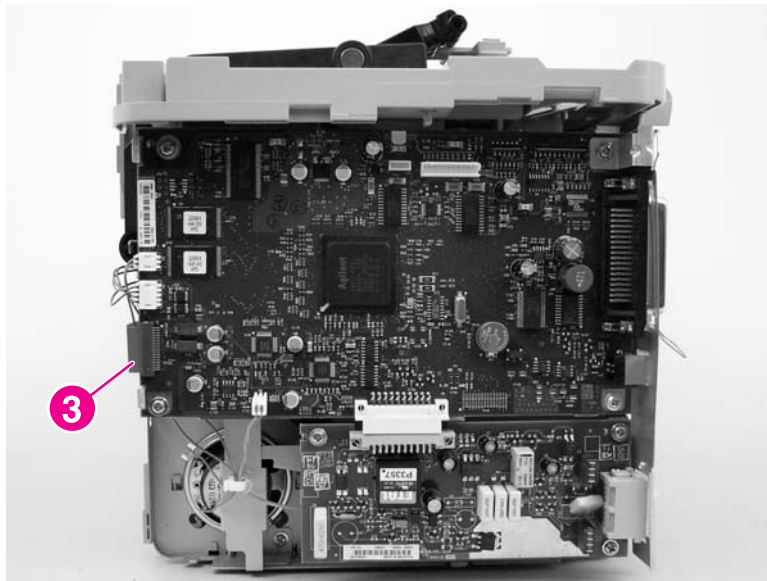
Figure 5-135. Remove the ECU (3 of 6)
